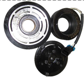
CL9303 SD7H15 6 RANURAS 12 VOLTS (125MM) P/COMP. 4792/ 4425/ 4424/ 4731/ 4815
